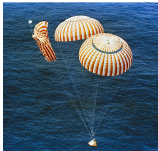
Apollo 15 Moon mission capsule during descent. One parachute failed on the way down.
