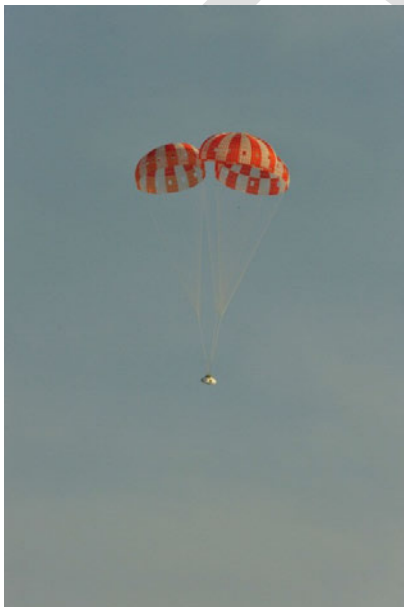
Orion capsule during a parachute drop test.
